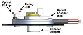
Optical Encoder Disk can not strke the Ignition Module or Optical Pickup at anytime during operation. Cam walk is normally outward so position Encoder Disk appropriately using shim washers.
