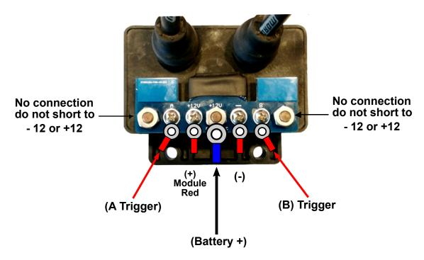
Remove the 3, 10-32 nuts and lock washers from the top of the SF coil terminals and place coil driver board on to coil as shown. Replace the 3, 10-32 nuts and lock washers with existing or new hardware supplied. Use appropriate #6 connectors for making terminations. Do not allow any of the connections to short to each other. See ignition wiring diagrams for wiring.
