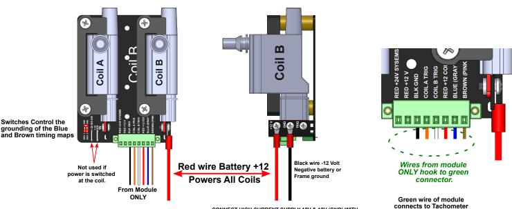
CONNECT HIGH CURRENT SUPPLY 12V & 12V (GND) WITH #6 RING CONNECORS TO TERMINAL SCREWS OF COIL B These connections supply power to both coils A & B
