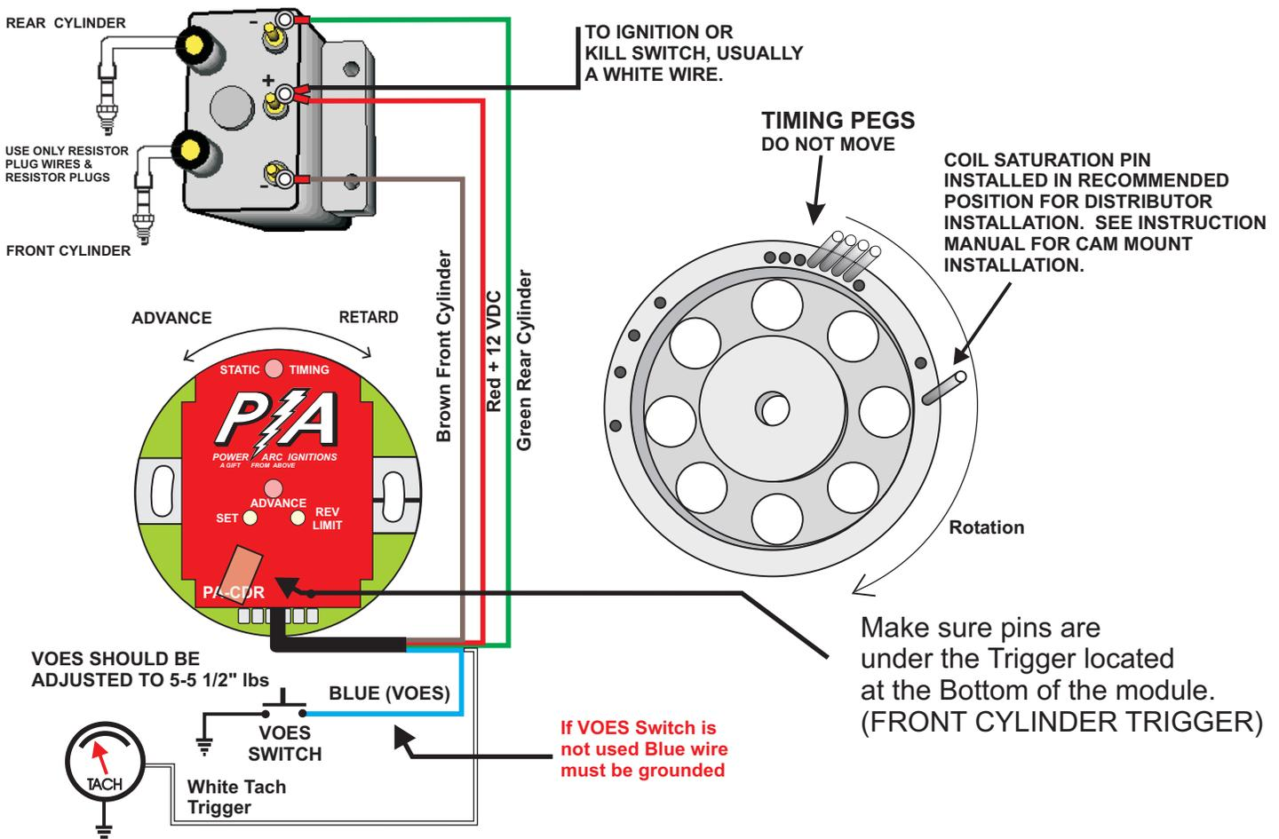
**Note:** Stock distributor will not work, a distributor that will accept cone mount ignition systems is required.
