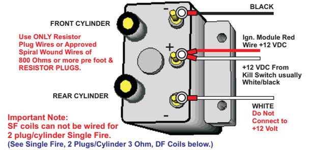
**Single Fire, 2 Plugs/Cylinder, 3 Ohm, DF Coils**
