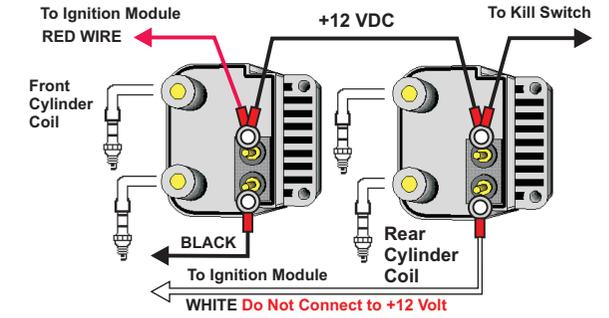
**Dual Fire, 1 Plug/Cylinder, 3 Ohm, DF Coil**
