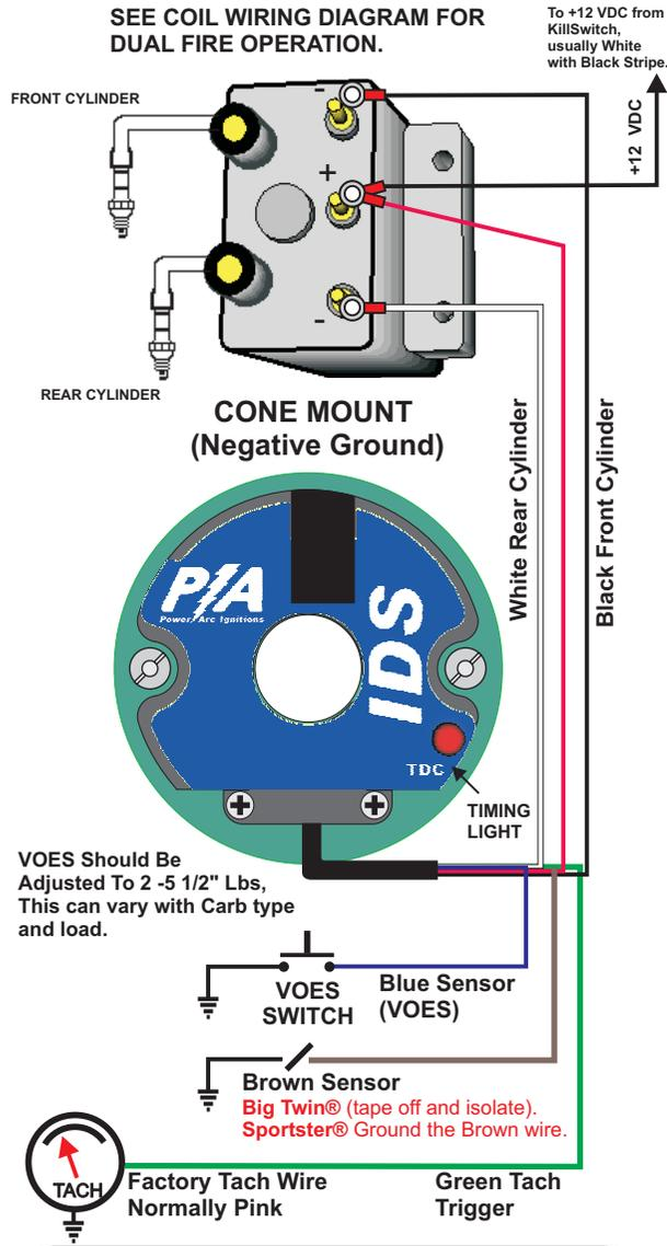
**WARNING: Do not touch coil output wires (White & Black) To +12. DO NOT USE SOLID OR SPIRAL WOUND SUPPRESSION SPARK PLUG WIRES. USE RESISTOR WIRES ONLY. FAILURE TO OBSERVE THESE PRECAUTIONS WILL DAMAGE IGN. & VOID THE WARRANTY.**
