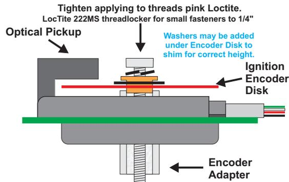
Extra washers may be included for shimming the Encoder Disk outward. Place on encoder standoff if Encoder Disk is too close to Optical Pickup.
